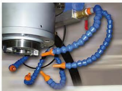
■ HIGH PRESSURE COOLANT WITH 4 WATER NOZZLES AND 1 AIR
