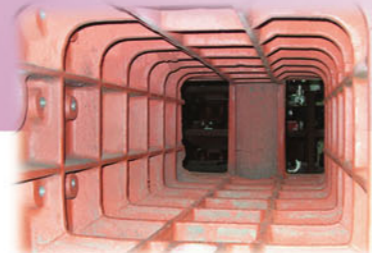
■ INSIDE CASTING CONSTRUCTION (RIBS) E422
